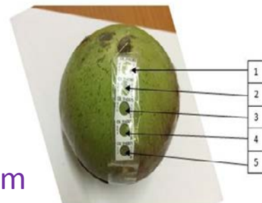
Hình 15: Dose distribution inside and outside star apple fruit
